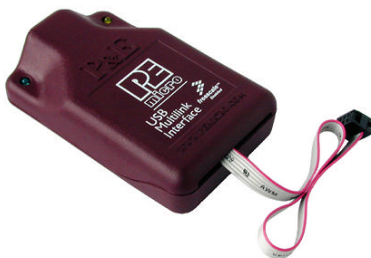
Figure 9-1: P&E's USB Multilink (USB-ML-12 shown)
