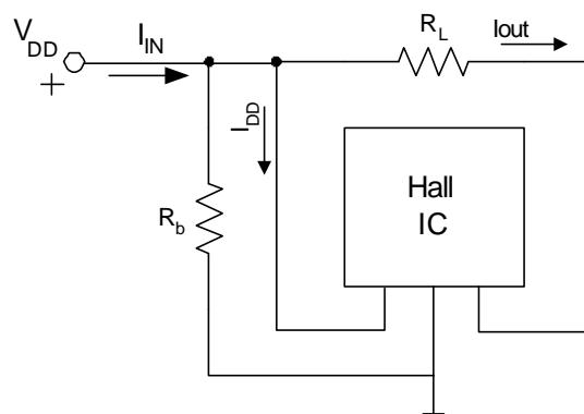
The resistors  $R_b$  and  $R_L$  can be used to bias the input current,  $I_{IN}$ . Refer to the part specification for limiting values. This circuit will help in getting the precise ON and OFF currents desired.
