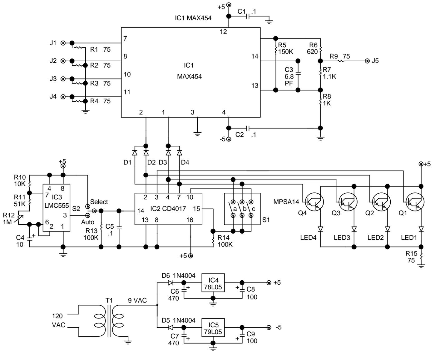
Fig. 1 The video switcher is built around a Maxim MAX454 multiplexer chip. Up to four cameras can be viewed on one monitor in sequence.
