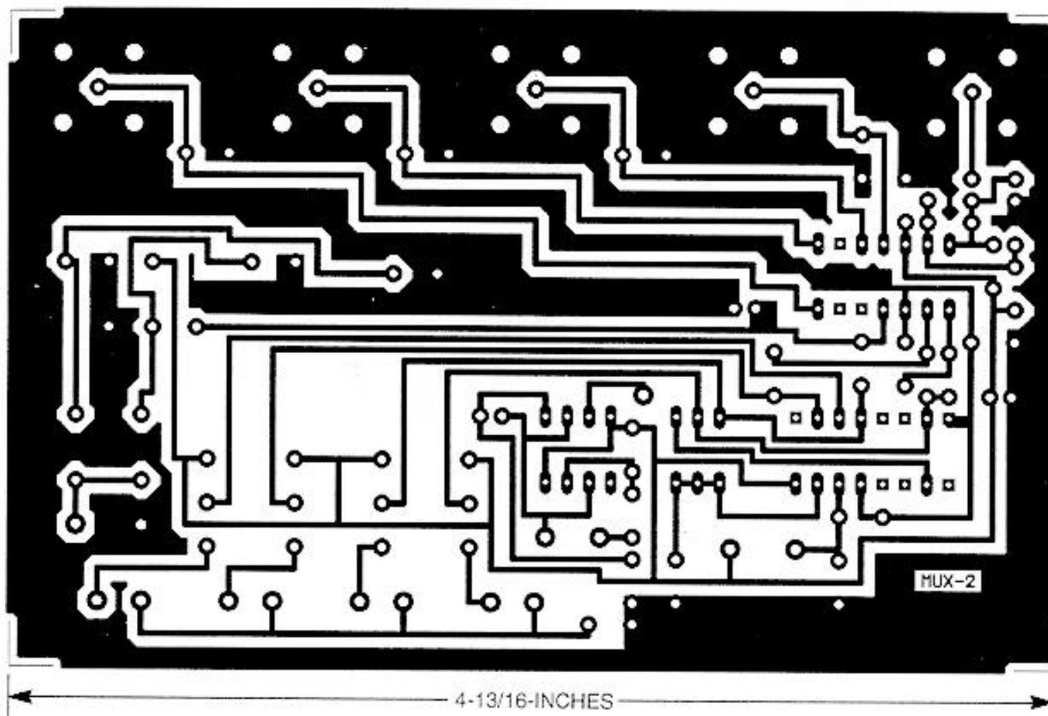
Here's the foil pattern for the video switcher. The circuit fits easily on a single-sided board. Ground traces around the video lines prevent noise and crosstalk.
