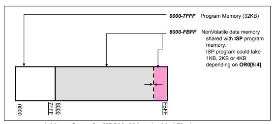
Address Space for MPC89x58A embedded Flash memory
